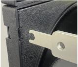
To gain access to the Light LED boards, use the custom tool provided by Data Signs.
