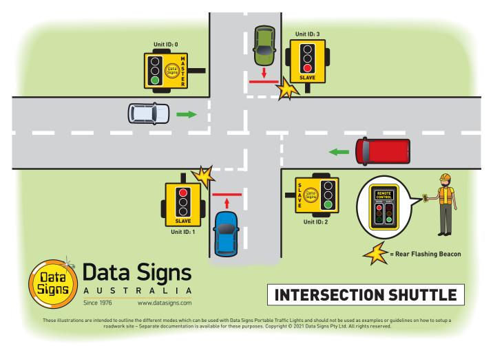
The Slave unit 2 (**Unit ID: 2**) will show the same signal light as the Master (**Unit ID: 0**). The Slave unit 3 (**Unit ID: 3**) will show the same signal light as the Slave (**Unit ID: 1**). The Manual, AUTO, and DEMAND modes are all available.
