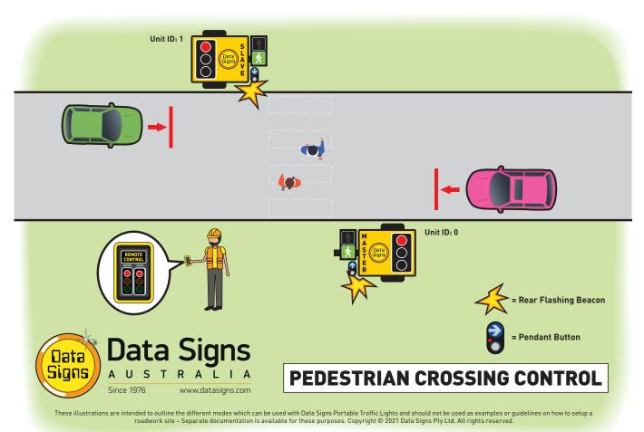
Once the physical installation of the Pedestrian Crossing Lights and Pendant Buttons is done on the PTL Set, use the **OPERATING SETTINGS** to select **PEDESTRIAN MODE**. Scroll down the Menu until **PEDESTRIAN** is displayed, then select **ENABLE**.
