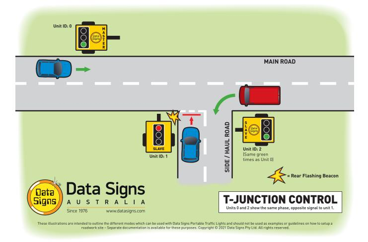
You can separate the green times using the button. Use the menu that appears to select each green time in turn. Unit 0 and 2 will use the same are time.
