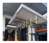
Each Traffic Light Trailer is fitted with a Directional antenna. This will provide reliable Wireless Radio (RF) communication between the PTL units; however, the units still need to be positioned line-of-sight to each other. The ends of each antenna should point *towards* the other. They can be adjusted on a swivel to help alight the correct direction.
